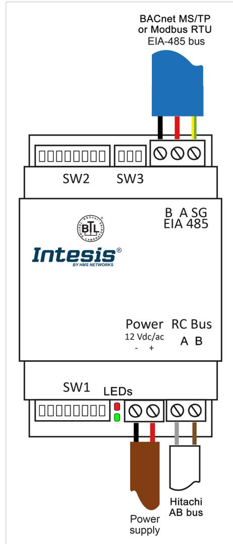
Figure 1. Wiring diagram (wire colors are indicative only)
